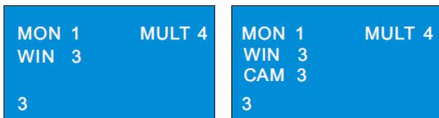
As a result, you will see the image of NO.3 camera in NO.3 window and 4 screens display mode will be seen in NO.1 monitor.
