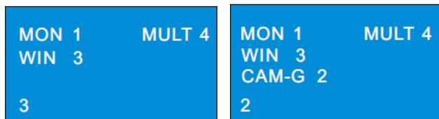
**Camera group settings:** go to TV wall client→Setup→Create Channel Group to create channel (camera) group and dwell time. Then click “Modify or Delete Channel Group” to add the channel for this camera group. The effective value is form 1 to 999999.
