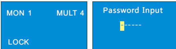
When the keyboard is locked, all keys except digital keys on the keyboard are unavailable until you input the password to unlock the keyboard.
