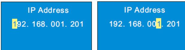
**Tips: Move the joystick right to set the IP address. Press “Enter” to save the settings and return to the previous menu.**
