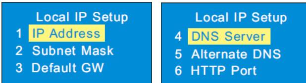
❖ IP address: Select IP address and press “Enter” to set the IP address. The default IP address is 192.168.1.201.
